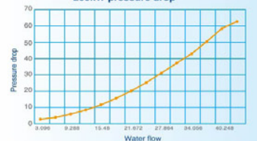
200kW pressure drop
